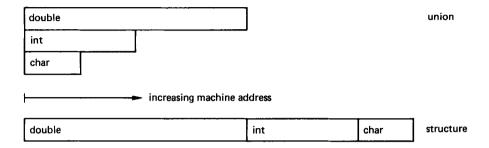
If we assume that the size of a char is 1 byte, of an int is 2 bytes, and of a double is 4 bytes, then the size of the union is 4 bytes, while the size of the structure is 7 bytes.
